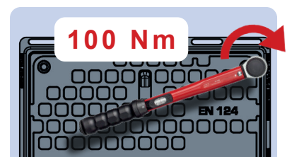
Fig. F: Tighten the bolts
